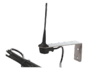
ANTS-433 Blade antenna to 433 MHz with steel bracket and RG-58 cable, L. 5000 mm
